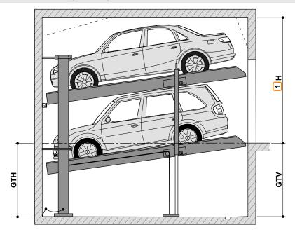
H: Ceiling height GTV: Pit depth, front GTH: Pit depth, rear
