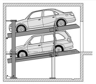
The lower vehicle can park in or leave the parking space. Incline of the lower platform approx. 8° = 14 %
