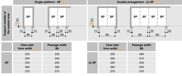
1 Door section (dimension A3 must be agreed on-site with the door manufacturer). With lateral closing doors, coordination between the door manufacturer and KLAUS Multiparking is required.
