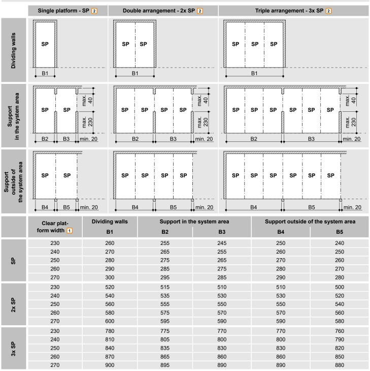
1 Narrower platform widths are available on request - although it should be noted that use of the parking space will be limited by the reduced width and parking will be made more difficult. In many cases, these are not considered demonstrable vehicle parking spaces - observe local regulations.
